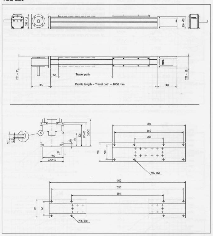
At the ends of the profile mechanical stops, cushions, are located 100 mm from the end surface. As precautionary measure there also is a safety distance between the carriage and the cushion when using the maximum theoretical travel path.
