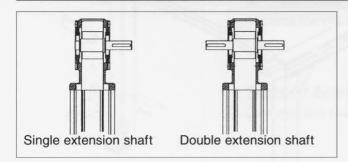
The units are primarily designed for fitting to hollow shaft transmission unit. Alternative models intended for transmission unit with extension output shaft and connection in series for multiple drive can be delivered. Units adapted to extension output transmissions are
